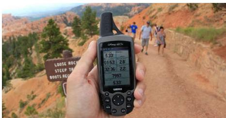
A GPS (Global Positioning System) device is a hand-held receiver that picks up signals from satellites circling the earth, enabling you to locate your current position to an accuracy of 10-20m. Most modern GPS devices can then show that position on a map and, if you have stored a pre-programmed route, help you navigate along it. For more information see Section 7 of the Guide for Leaders on the Lancaster RA website (<http://www.lancasterramblers.org.uk>).
